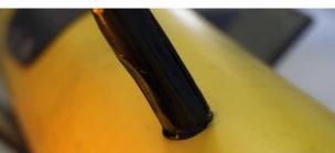
**Kebu Meltstick** is ideally suited for repairing the factory coating if the damage is superficial and if it does not exceed a size of 10mm. It's compatible with factory coatings made of PE, PP, FBE, PU and Bitumen.
